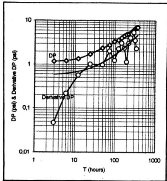
Figure 8. Plot of Pressure and Derivative Pressure DRJ#S<sub>1</sub>
