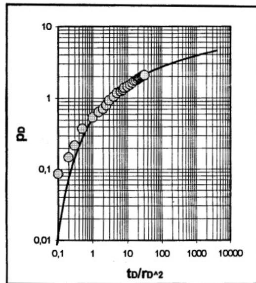
Figure 10. The Type Curve Matching of DR#S<sub>1</sub> Using Conventional Type Curve
