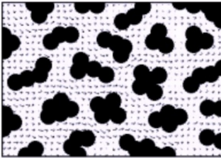
Figure 7. The simulated fluid flow in porous medium for 24.810% porosity.
