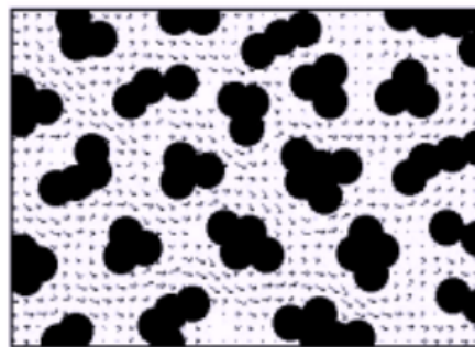
Figure 6. The simulated fluid flow in porous medium for 29.837% porosity.
