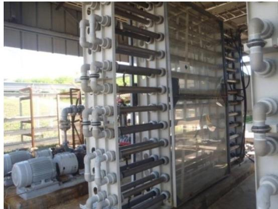
**Gambar 9. Rangkain Alat Unit Electrochlorination**
