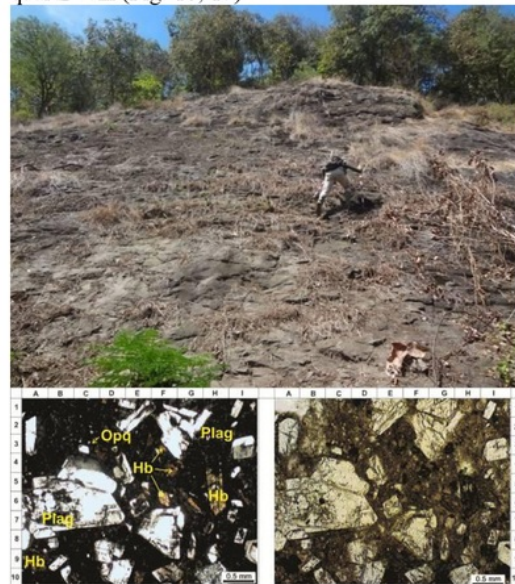
Fig.15: Hornblende andesite lava at Mt. Butak (upper), and its petrographic analysis (lower)
