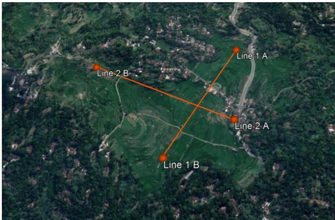
Gambar 4. Lintasan pendugaan geolistrik metode Dipole dipole. (sumber peta; google earth).
