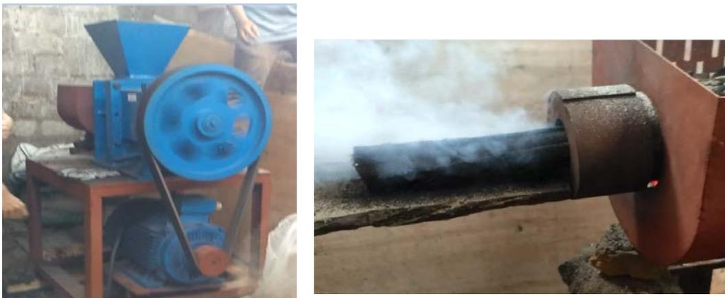
Gambar 2 (a) Mesin heated die screw extruder, (b) Proses pembriketan
