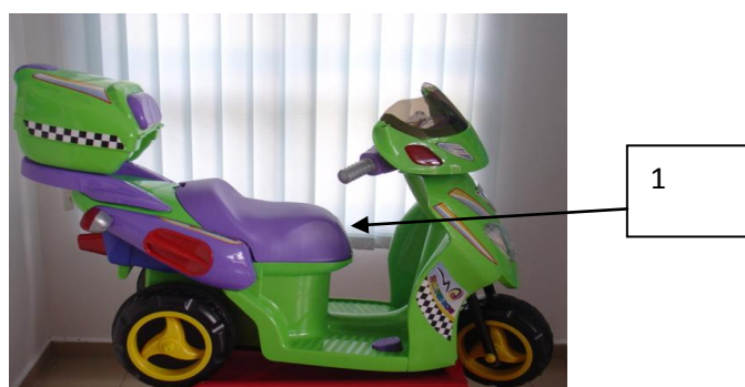
Figure. Chem –E-Car 60 Watt, Fuel Cell powered demonstration Car (SERINDIT).
