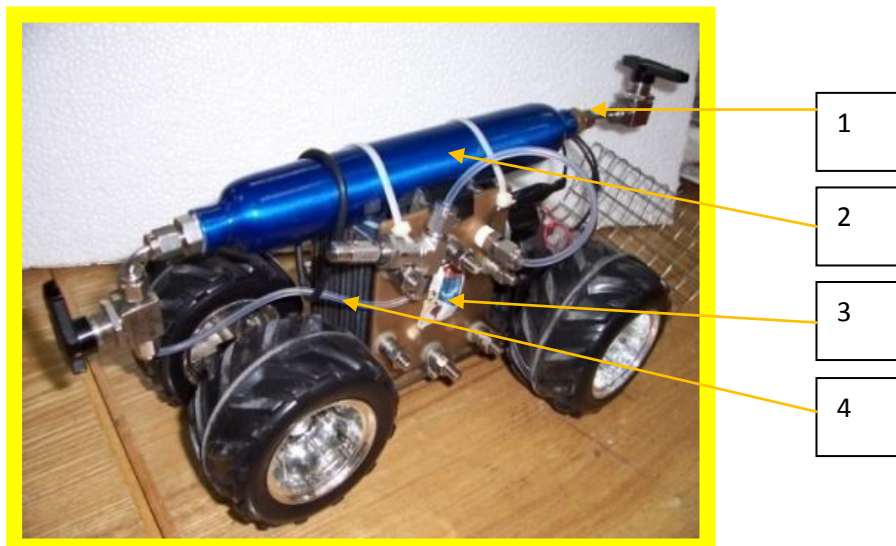
Figure. Chem –E-Car 10 kW, Fuel Cell powered demonstration Car. (1) Hydrogen feed storage feed, (2) Storage Hydrogen , (3) PEM Fuel Cell 10 Watt, (4) Pipe
