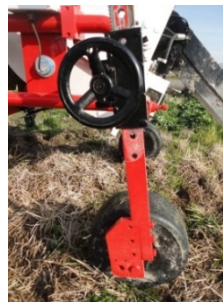
Figure 3. The gage wheel on both sides of RTSS can be adjusted of 5 cm spacing to collect soil spectra at the depth of 5cm to 35 cm from the topsoil.
