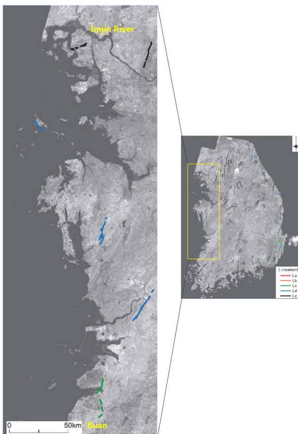
Fig. 5 Lineament map interpreted by ASTER image around the western part of the Korean Peninsula.
